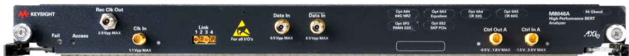
Figure 12. Front panel views of pattern generator module M8045A (top) as 2 and 1 channel (center) versions, remote head M8057A/B, and error analyzer module M8046A (bottom). To allow a very short connection to the device under test, the remote head is used. One remote head is needed for each of the pattern generator data outputs of M8045A.
