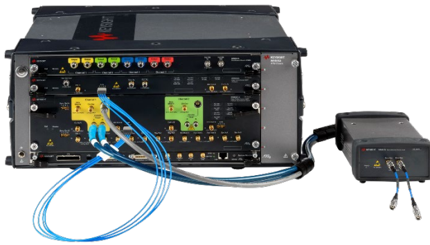
Figure 3. The remote head M8057A/B is required for each channel and is required for NRZ and PAM4 signals. It contains an adjustable gain amplifier without re-timer. Users can select NRZ or PAM4 coding and de-emphasis taps settings from the user interface with no need to reconnect cables. The cable between the remote head and the module is 0.85 m long. This allows positioning the remote head closely to the test board for the device under test.
